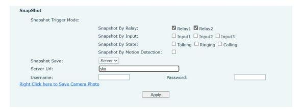
(2) After the setting is completed, the door is opened by webpage, card, password and other door opening methods to trigger the door capture, and the captured pictures will be uploaded to the configured server.
