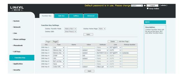
Configure the DSS Key on page N, set a softkey or navigation key to Dsskey PageN, press the softkey / navigation key of the corresponding interface, enter the Dsskey Page, select a DSS Key, or press the corresponding serial number of the DSS Key to perform the corresponding function.
